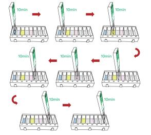
10. Pick up the Solid Array Unit and insert it into the compartment 6, and let it stand there for 10 minutes..
